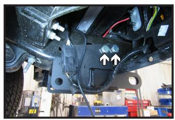
3. Slide baseplate onto the frame with convenience link towards the center of the vehicle until the holes line up with the two (2) existing holes in the frame. Insert the two (2) 5/8" x 6-1/2" bolts into the holes to hold the baseplate in place. Do this on both sides of the vehicle.
