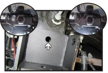
4. Install the 5/8" x 1-3/4" bolt with lock washer into the indicated hole and insert 5/8" wire nut as shown in insets. Do this on both sides of the vehicle.
