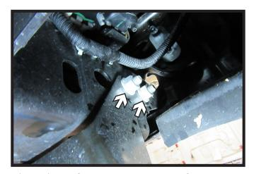
2. Using an 18MM socket, remove the four (4) nuts (white) and factory bolt hardware from the bracket. Do this on both sides of the vehicle. Remove brackets and set aside. They will not be reinstalled.
