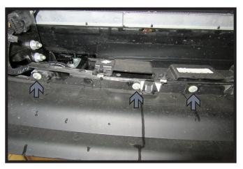
1. Using an 8MM socket, remove the thirteen (13) bolts from the lower bumper valance. There are three (3) bolts (white) on each end that are accessible from above and the other seven (7) bolts (gray) are accessible from below. Remove valance and set aside to be reinstalled later.
