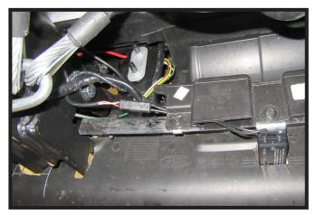
Holding the bumper valance as close to original position as possible, mark and trim necessary clearance for baseplate and optional breakaway switch.
