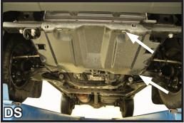
1. Using a 12MM socket remove the four (4) bolts, two (2) per side, from the belly pan and set aside for reinstalling after baseplate installation. NOTE: Some models may not have a belly pan.
