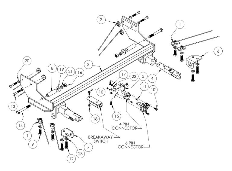
NOTE: Items #7 and #8 need to be rotated 180° for 2011-2012 models so the holes face inward. Remove existing tie down brackets prior to installing the convenience links that have been supplied with your baseplate.
