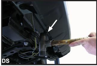
Remove the two (2) push pins from the bottom edge of the front fascia. After removing the push pins, use a rubber mallet to bend the tabs upward where the push pins were located. This will prepare the opening for the baseplate installation.
