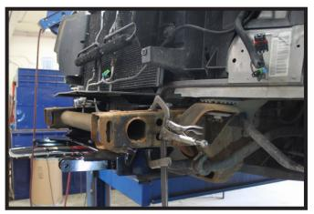
Position the baseplate onto the frame, lining up front hole on the underside of the frame and the back hole of the baseplate. Square and clamp the baseplate securely to the frame.
