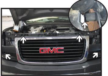
3. Using a 10MM socket, remove the four (4) screws from the grille. There are two (2) on each side.
