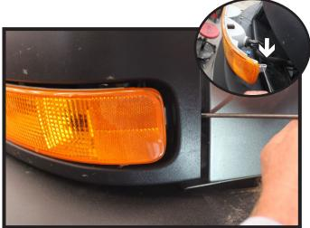
2. Using a flat screwdriver, pry behind the grille to release the clip and release the park light from frame. Disconnect all electrical connections and set aside. Do this on both sides of the vehicle.
