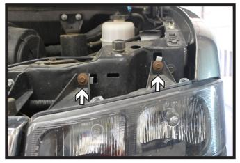
Using a 10MM socket, remove the two (2) screws from the headlight. Disconnect all electrical connections and set aside. Do this on both sides of the vehicle.
