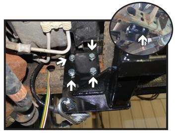
Continue drilling the remaining holes in the baseplate thru the frame. Install 1/2"-13 x 1-1/2" bolts with lock washers into the holes and a 1/2" whiz nuts on the inside of the frame. Do this on both sides of the vehicle. Fully tighten all hardware.
