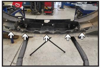
8. Remove the five (5) push pins from the lower valance on the bumper. The valance will not be reinstalled for baseplate clearance.
