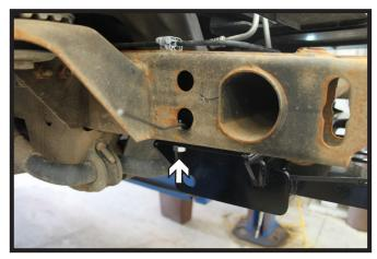
Using a 17/32" drill bit, ream out the bottom back hole. Install a 1/2"-13 x 1-1/2" bolt with lock washer into the hole and a 1/2" whiz nut on the inside of the frame. Do this on both sides of the vehicle. Fully tighten all hardware.
