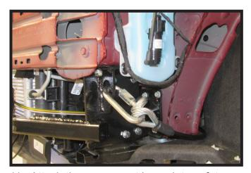
11. Attach the permanent baseplate safety cables to the provided convenience link on the baseplate. The photo above shows the recommended installation of the cables to frame of vehicle. Additional options may interfere with suggested mounting; in this case, secure the cables to a solid piece of the frame as described in the General Information sheet. Be sure the safety cables do not rub against any hoses or moving parts. Do this on **BOTH** sides of the vehicle.
