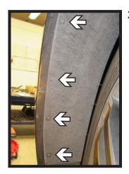
Using a T15 Torx, remove the four (4) screws from the wheel well in front of the tire. Do this for both sides of the vehicle.
