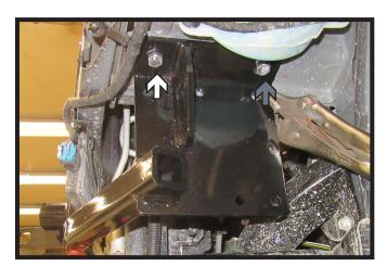
7. Slide the baseplate on and clamp into place. Install the provided 3/8" hardware into the existing holes on both sides of the vehicle (white). Using a 3/8" drill bit, drill out the back holes (gray) and install the 3/8" hardware.
