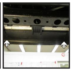
5. Using a 7MM socket, remove the ten (10) bolts from the underside of the car. There are three (3) in front of each tire, two (2) on each side of center, and two (2) in the center.
