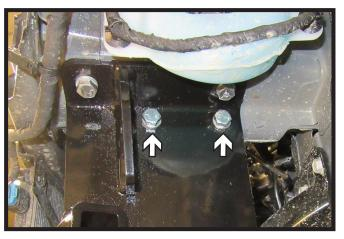
8. Using a 3/8" drill bit, drill out the holes on both sides of the baseplate, and insert the provided 3/8" hardware.
