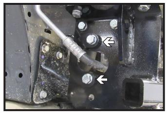
On the passenger side, attach the reinforcement brace around the line. Install with the provided 3/8" hardware.
