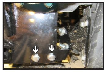
Secure U-bolt around the frame extension behind the baseplate, and install to baseplate with the provided brace and associated 3/8" hardware.
