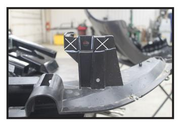
12. **2014 Models:** Remove the two (2) screws from the plastic shroud and trim the outer portions for baseplate clearance. Do this on both sides of the shroud and reinstall.
