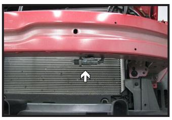
2011-13 Models: Remove the temperature sensor from the bottom of the bumper on the driver's side.
