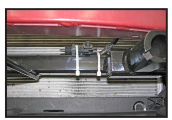
16. **2011-13 Models:** Attach the temperature sensor to the baseplate crosstube with zip ties.
