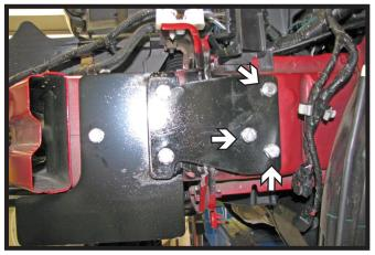
15. Using a 13/32" drill bit, drill the three (3) holes thru the frame. Install 3/8"-16 x 2" bolts with 3/8" lock washers into the holes and 3/8"-16 nut plates on the inside of the frame. Do this on both sides of the vehicle. Fully tighten all fasteners.
