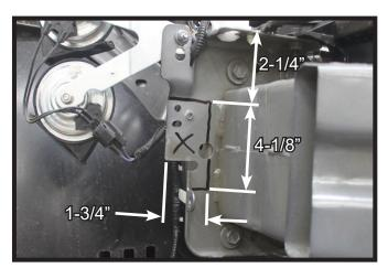
8. Using a reciprocating saw, trim the face of the frame as shown for baseplate clearance. Do this on both sides of the vehicle.
