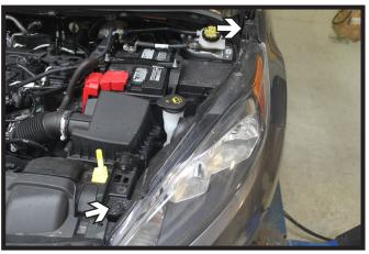
5. **2014 Models:** Using a T30 Torx, remove the two (2) screws from the headlight. Disconnect the electrical line and set the head light aside. Do this on both sides of the vehicle.
