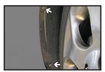
2. Using a T25 Torx, remove the two (2) screws from the wheel well. Do this on both sides of the vehicle.
