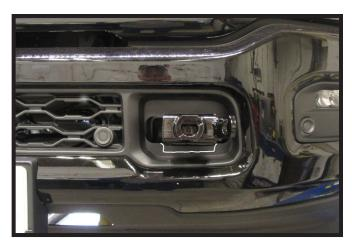
3. Slide baseplate into tow hook housing as far as possible. Mark plastic for trimming. Do this on both sides of the vehicle.
