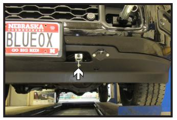
8. **Optional Breakaway**: Using the provided 1/4" hardware, attach the breakaway switch to the vehicle bumper as indicated.
