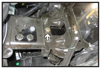
Slide baseplate into place. Insert one (1) 5/8" x 3-1/2" bolt into the existing hole.
