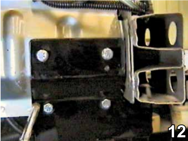
12. Using the baseplate as a template, drill the four holes on the passenger's side and three holes on the driver's side with the 13/32" drill bit.
