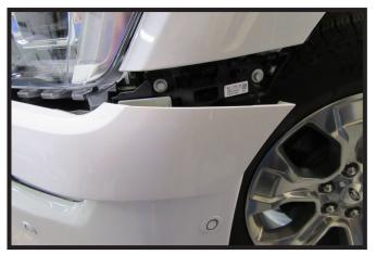
4. Remove the middle fascia piece by grabbing the edge and pulling outward. Set piece aside to be reinstalled later.
