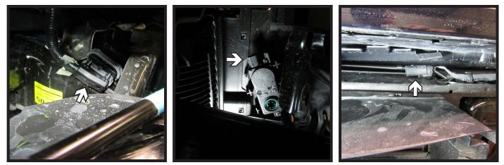
2. Start to remove the bumper. As the bumper is removed unplug the main electrical (left) and shutters (center) from passenger side of the vehicle. Then unplug electrical on top of the shutter housing (right) on the driver side of the vehicle. Set bumper aside to be reinstalled later.
