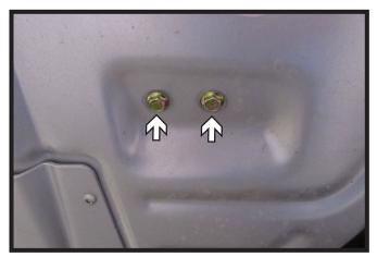
8c. **Raptor Models:** Use the four (4) provided shorter M10 bolts to reinstall skid plate. Reinstall the bumper and reconnect all electrical connections.
