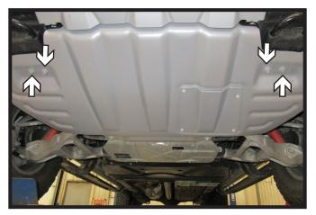
Using a 13MM socket, remove the four
