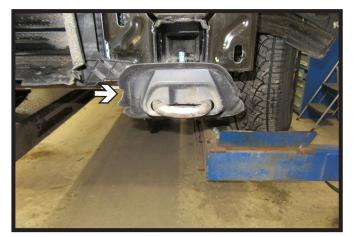
1. Remove the rubber piece from the tow hook. Do this on both sides of the vehicle.
