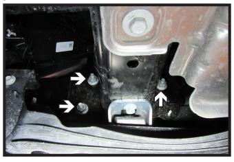
Using a 21MM socket, remove the three (3) nuts from behind the bumper. Do this on both sides of the vehicle.
