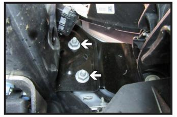
Coming from underneath the vehicle, use a 21MM socket to remove the two (2) outer nuts from behind the bumper. Do this on both sides of the vehicle.
