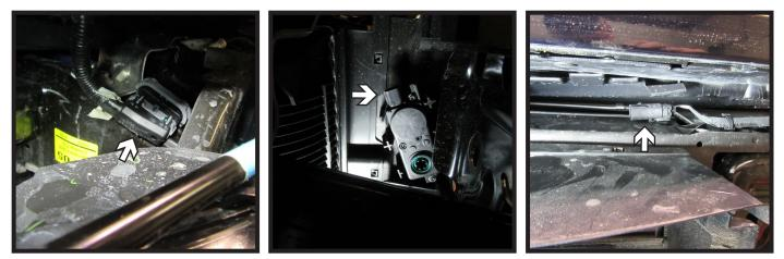
5. Start to remove the bumper. As the bumper is removed unplug the main electrical (left) and shutters (center) from passenger side of the vehicle. Then unplug electrical on top of the shutter housing (right) on the driver side of the vehicle. Set bumper aside to be reinstalled later.
