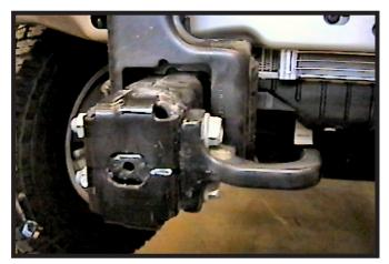
Remove two (2) bolts from the tow hook using the 18MM socket. Do this to both sides of the vehicle.
