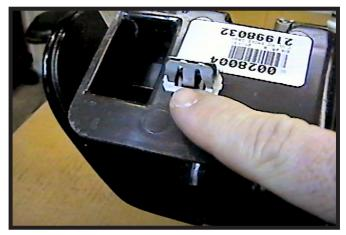
4. Remove all seven metal clips from the metal frame and reinstall them to the tabs on the back side of the grille.
