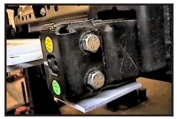
Hold up the baseplate up and align with the existing tow hook holes. Insert 1/2"-13 x 3-1/2" bolts into the holes. Be sure that baseplate is level with the vehicle and temporarily tighten with a nut.
