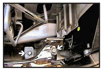
Using the 15MM socket, remove two (2) bolts from the top side of the metal bumper, just inside of the headlight assembly. Do this to both sides of the vehicle.
