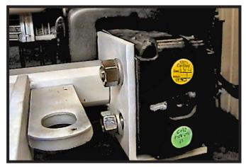
Remove the four (4) hex nuts from the 1/2" x 3-1/2" bolts. Install lock washers and fully tighten all fasteners.
