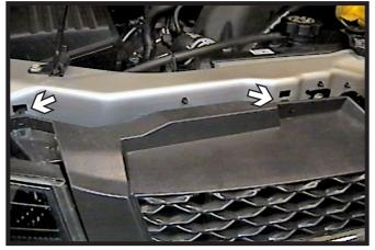
1. Push down on the four (4) retainer clips to release the grille.
