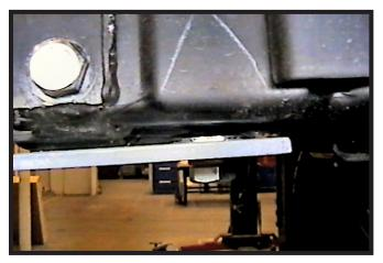
Using the baseplate template, drill the lower hole into the frame with the 17/32" drill bit. Do this to both sides of the vehicle. Loosen bolts installed in Step 9, slide the 1/2" flat washer between the frame and the baseplate to align with the drilled hole.
