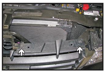
Using a 10MM socket remove two bolts from the top front edge of the grille. Do this to both sides of the vehicle.
