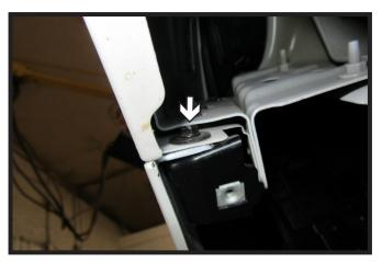
Carefully pull back wheel well liner. Using a 7MM socket, remove the one (1) bolt. Do this on both sides of the vehicle.
