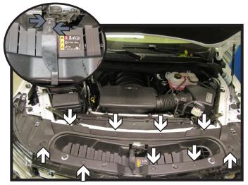
Remove the nine (9) push pins (white) from the fascia cover. Using a T15 Torx, remove the two (2) screws from the hood latch handle (inset gray). Set aside the facia cover and hood latch handle to be re-installed later.
