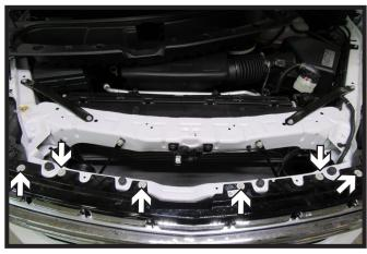
2. Using a 10MM socket, remove the six (6) bolts from top of facia.
