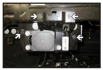
9b. **Models With ACC**: Using a 7MM socket, remove the four (4) mounting bolts from the ACC and allow to hang out of the way. This will be re-installed later.
