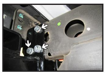
13. Slide baseplate back into place. Using one (1) 1/2" bolt on each side, insert into an existing hole to hold in place. Again, clamp baseplate firmly against bottom of frame on both sides. Install three (3) 1/2" x 1-1/2" bolts with lock washers and wire nuts in the side mounting holes. Tighten fully. Do this on both sides of the vehicle.
