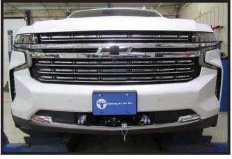
17. Hold the fascia as close to its original position as possible. Mark and trim the fascia as needed for clearance with the baseplate components. Reinstall the fascia and fascia covers.
