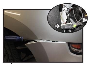
7. Gently pry the fascia loose from the front end. Carefully unplug two (2) electrical connections on the passenger side behind the facia (inset). Remove the fascia from the vehicle and set aside.
