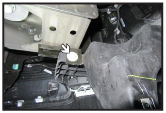
6. Using a 10MM socket, remove the one (1) bolt. Do this on both sides of the vehicle.
