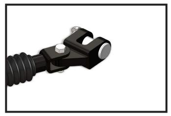
2. Install the offset double lug onto the tow bar leg with the new washers, 1/2"-13 x 2" bolt and 1/2"-13 jam nut provided. Tighten the bolt until the lug is tight against the washers, but can still freely move side to side. Do this on both tow bar legs.
