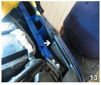
13. DODGE ONLY: Using a flat screwdriver, pull plastic forward to loosen. Do this to both sides of the vehicle. The bumper and grille can then be removed and carefully set aside to be reinstalled later.
