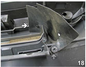
18. DODGE ONLY: Remove rubber piece from the backside of the fascia, by first removing the pushpin with a flat screwdriver (white arrow) and then cutting right next to the clip with a utility knife (gray arrow). The rubber piece should be completely removed and discarded. Do this to both sides of the fascia.
