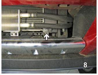
3. JEEP ONLY: Using a flat screwdriver in front remove two more push pins, one on each side. (Some models may have three pushpins.) Pull fascia corners out to the side and then forward to release. Set fascia aside carefully to be reinstalled later. (JEEP: Go to Step 14)
