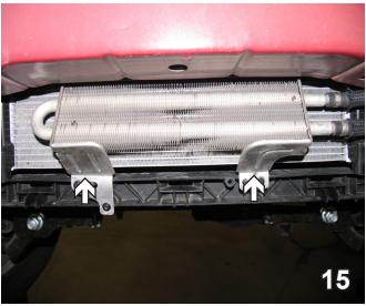
15. **JEEP ONLY:** Under the transmission cooler, bend the brace brackets up to 45°. Being careful not to damage radiator behind transmission cooler.
