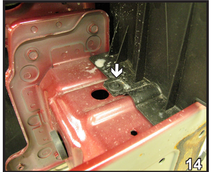
14. On the passenger side, remove the push pin from the top of the air dam. Do this to both sides.
