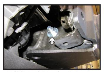
3b. **Baseplates Made After (4/12/23)**: Install the one (1) 1/2" bolt with flat washers, lock washer, and nut. Do this on both sides of the vehicle.
