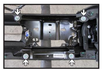
Using a 13MM socket, remove the four
