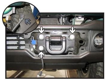
Using a 15MM socket, remove the three
