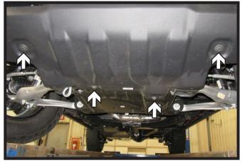
Using a 15MM socket, remove the four
