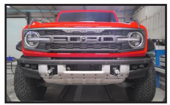
9c. Reinstall belly pan. Hold tow hook cover as close to its original position, mark and trim the covers as needed. Reinstall bumper cover.
