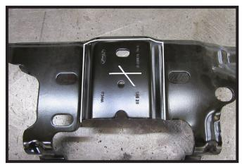
Using a reciprocating saw, cut and remove the indicated area of the tow hook bracket. Do this on both D-ring brackets. Reinstall brackets onto bumper.
