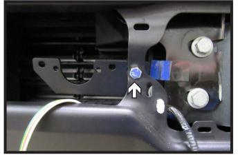
8. Hold electrical bracket up to the bumper on the driver side of the baseplate and mark spot. Using a 1/4" drill bit, drill a hole in the bumper. Attach bracket to the bumper using one (1) 1/4" x 1" bolt with flat washer and nylon lock nut.
