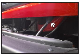
3. **Raptor Models**: As the bumper is removed, unplug the one (1) electrical connection on the driver side of the vehicle
