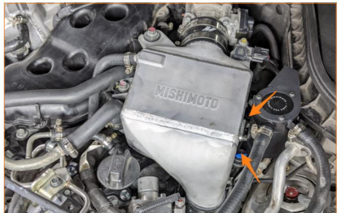
**04.** Reinstall hoses and tighten clamps.
