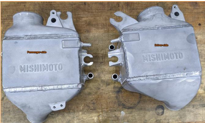
11. Install brackets onto intercoolers using supplied M6 bolts.
