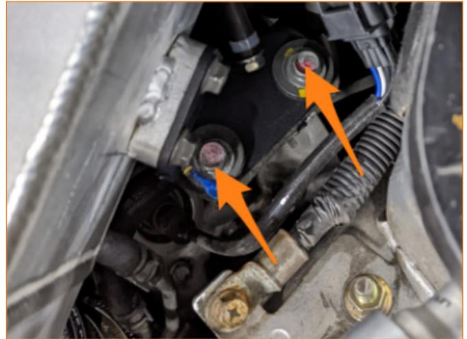
**03.** Install catch can bracket over Intercooler bracket and reinstall bolts holding both brackets down.
