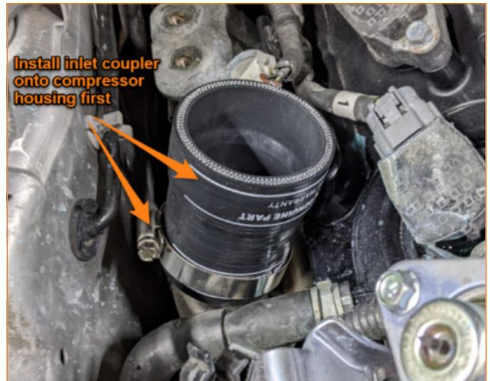
16. Place inlet of intercooler into inlet couplers first.
