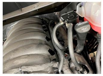
**9.** Adjust the catch can in the slotted holes, ensuring that it clears the engine oil fill cap and none of the hoses are kinked. Tighten the 3x bolts with a 2.5mm allen key.
