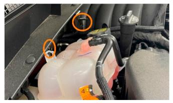
6. Install the catch can and bracket assembly onto the two studs on the firewall behind the coolant reservoir. Secure with the two included 10mm lock nuts. Reinstall the coolant reservoir with the factory 10mm bolt.
