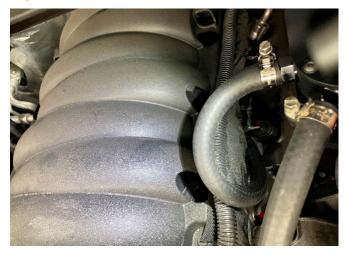
8. Take the hose with the straight fitting and install the quick connect fitting to the fitting on the valve cover. Attach the open side of the hose to the "IN' fitting on of the catch can and secure with included worm gear clamp. The worm gear clamp is optional and the catch can will function leak free without the clamp.
