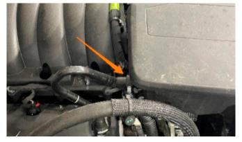
2. With a 7mm socket or flathead, loosen the 2x clamps on the intake assembly. The first clamp is located behind the mass air flow sensor and the second clamp is located at the throttle body. Remove the intake from the throttle body and mass air flow sensor and rotate the intake assembly counter-clockwise out of the way.
