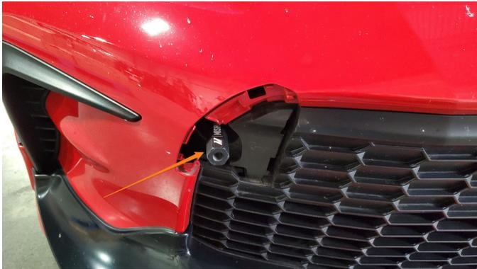
**05.** Using a 16mm socket, attach the license plate bracket to the rod with the supplied M10 hex head bolt & washer.
