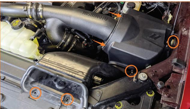
13. Secure the coolant hose to the Mishimoto intake tube with the provided tree clip zip tie.
