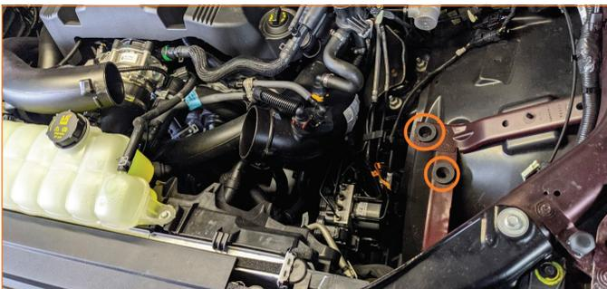
**5.** Install the 2x brackets and 2x pegs onto the Mishimoto intake airbox, as shown in the pictures below. Use the two larger M6 flat washers on the pegs.
