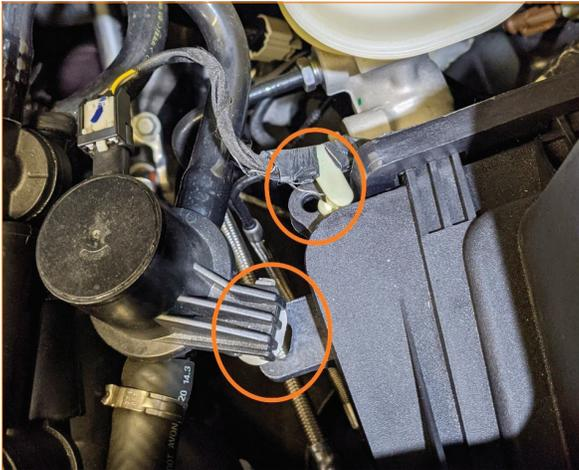
**4.** Lift the airbox straight up to disengage the 2x rubber grommets. Remove the stock airbox from the vehicle.
