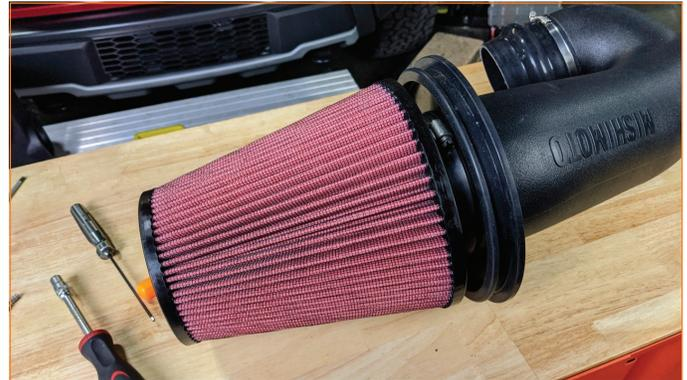
**7.** Transfer the IAT sensor from the stock intake tube to the Mishimoto intake tube. Attach the 2x silicone couplers to the intake tube, secure with 2x worm gear clamps (7mm socket).
