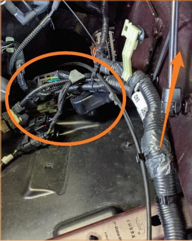
9. Install the airbox assembly first, engage the bottom pegs into the rubber grommets in the engine bay and adjust the harnesses mentioned in step 8 if needed.
