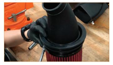
**11.** Assemble the passenger-side air intake by inserting the tube assembly into the airbox. Push the rubber grommet lip all the way around to fully seat it in the airbox lip.
