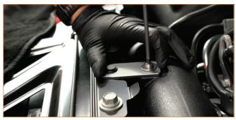
**24.** Reinstall the engine cover and strut braces. The strut brace nuts should be torqued to 28Nm (21 lb-ft). The bolt should be torqued to 56Nm (41 lb-ft).
