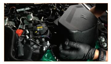
**17.** Install the CNC aluminum adapter onto the plastic driver side turbo snout. Ensure the spring clip is properly seated before pushing down on the adapter to engage the clip.
