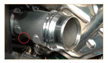
**05.** Remove the two pop clips securing the driver-side intake tube to the radiator support bar.
