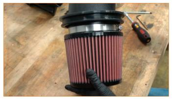
**14.** Assemble the driver side air intake by inserting the tube assembly into the airbox. Push the rubber grommet lip all the way around to get fully engage it into the airbox lip.
