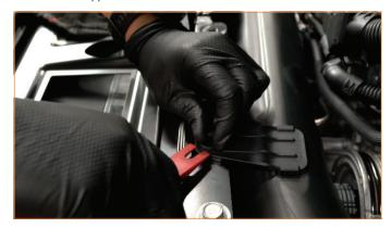
**06.** Loosen the worm gear clamp securing the driver-side intake to the airbox. Separate the intake tube and the air box, then lift the air box straight up to disengage the rubber grommets and remove them from the engine bay.
