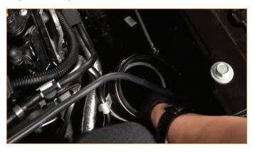
**19.** Temporarily disconnect the electrical harness shown to gain more clearance when installing the driver-side intake.
