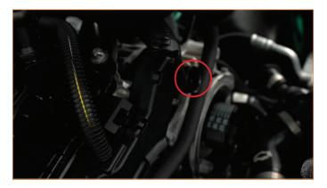
**20.** Install the driver-side intake assembly. Line up the intake tube with the silicone coupler, then push down on the airbox to engage the bottom rubber grommets.
