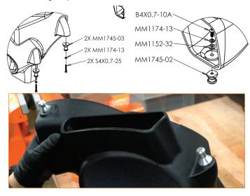
**10.** Identify and assemble the passenger-side intake tube, rubber grommet, and air filter as shown. Use the air filter with a smaller inlet diameter and the smaller rubber grommet in the kit. Ensure the air filter is properly seated, then tighten the worm gear clamp.
