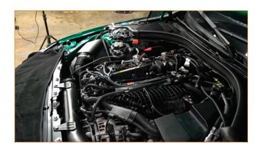
**02.** Remove the passenger-side intake. Loosen the worm gear clamp securing the intake tube to the airbox. Separate the intake tube and the air box, then lift the air box straight up to disengage the rubber grommets and remove the stock airbox from the engine bay.
