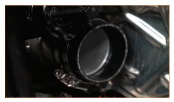
**16.** Install the passenger-side intake assembly. Lower the tube side into the engine bay first and align the intake tube with the coupler, then push down on the airbox to engage the pegs with the rubber grommets. Tighten the other worm gear clamp to secure the intake tube to the silicone coupler.
