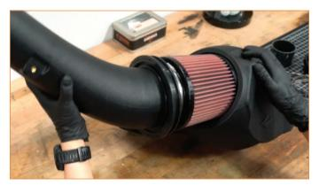
**15.** Install the straight silicone coupler to the Mishimoto aluminum turbo snout with 2x 50-70mm worm gear clamps. Tighten one of the worm gear clamps to secure the coupler to the turbo snout, leave the other one loose.
