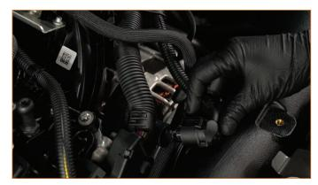
22. Tighten the remaining worm gear clamp.
