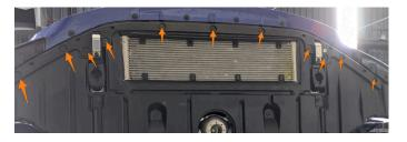
**02.** Remove the remaining bolts holding the center splash guard and remove. (Image on right)
