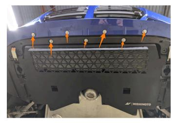
**06.** Hand tighten the stock bolts in the remaining mounting points, once all bolts are started torque all bolts down.
