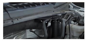
**15.** Attach the 3oz catch can to the bracket using the hardware in your kit. (3x 2.5mm Allen bolts)
