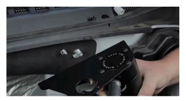
14. Secure the bracket to the firewall. Place the ground strap back over the stud, and then set the bracket over the two studs.(1x 15mm acorn nut, 1x 10mm nut and washer)
