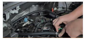
**06.** Run both hoses along the back of the engine.
