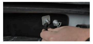
11. Connect MM4652-04 to the OUT port on the 12oz catch can.(1x worm gear clamp)
