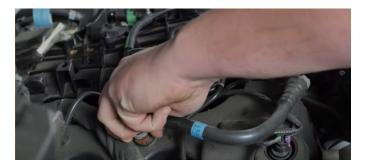
**04.** Connect MM4652-04 to the intake manifold. Slide the green tab down to secure the connection
