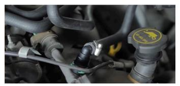
10. Remove the nut that secures the ground strap to the firewall.Then slide the plastic prop and metal plate off the nearby stud.(1x 15mm acorn nut)
