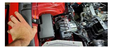
**11.** Install the straight end of the hose that was assembled in step 3 onto the PCV valve and secure with (1) supplied 20-32mm worm gear clamp. A 7mm socket, swivel adapter, and extensions may be needed to reach the worm gear clamp to tighten.
