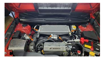
**05.** Remove the OEM PCV to intake manifold hose using pliers to loosen the (2) spring clamps. Long reach needle nose pliers and/or a remote-action hose clamp tool will make this much easier.
