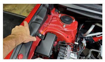
**08.** Using a 12mm socket, remove the bolt from the stud shown in the photo below.
