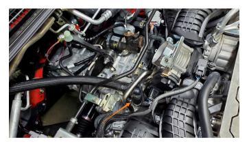
12. Install the larger end of the supplied bent hose onto the intake manifold and secure with (1) supplied 20-32mm worm gear clamp. Note: do not remove the permanent clamp that is preinstalled onto this hose. This clamp secures the internal spring to prevent it from entering the intake manifold.
