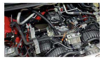
13. Install the hose from the intake manifold, that was just installed in step 12, onto the catch can port labeled "OUT" and secure with
