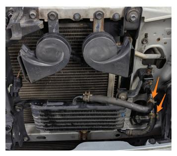
3. Remove the four M6 bolts holding the transmission cooler.
