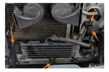
**4.** Remove the M8 bolt from the left horn bracket. Then unclip the ambient temperature sensor from the radiator support. Let both items hang loose for now.
