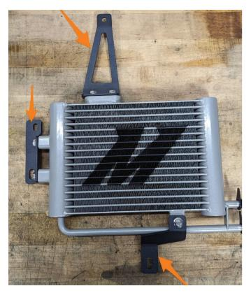
**6.** Install the transmission cooler using the supplied M8 and M6 bolts as shown. Make sure the top transmission cooler bracket goes behind the horn bracket. Tighten all hardware. (Image on next page)
