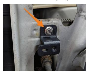
Bolt the hard transmission lines to the bracket using the shorterM6 bolt.
