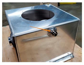
04. Ensure the outer clamping nut on the bulkhead is loosened and feed the pump's wires from the inside of the tank through the holes in the bulkhead. Then, using a 22mm wrench, tighten the outer clamping nut to seal the bulkhead around the wires.
