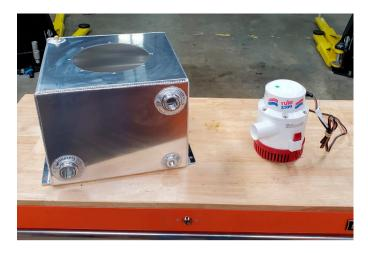
O1. Remove the strainer basket from the pump and, using a 2.5mm Allen wrench and the [4] supplied M4 bolts, lock washers, and flat washers, install it inside the tank in the orientation shown in the photo below. On the 5.0 gal tank, the outer holes will be used to mount a Rule 3700 pump and the inner holes will be used to mount the Rule 2000 pump.
