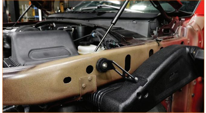
14. Reverse steps 5-9 and reinstall the headlight, fender headlight bracket and trim piece. Check to make sure the drilled holes on the fender line up with the threaded holes on the Borne Off-road snorkel fender tube.
