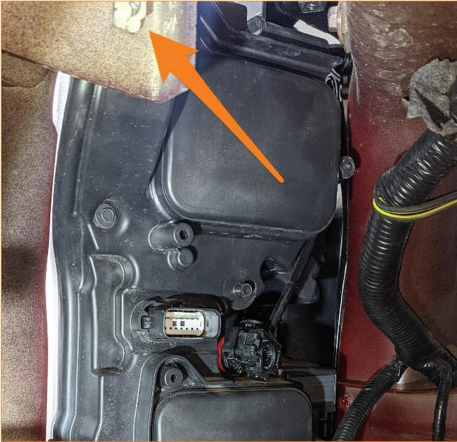
10. Modify the fender to install the Borne Off-Road snorkel fender tube. Follow the instructions on the template and reference the full install video on Mishimoto YouTube channel for more details.
