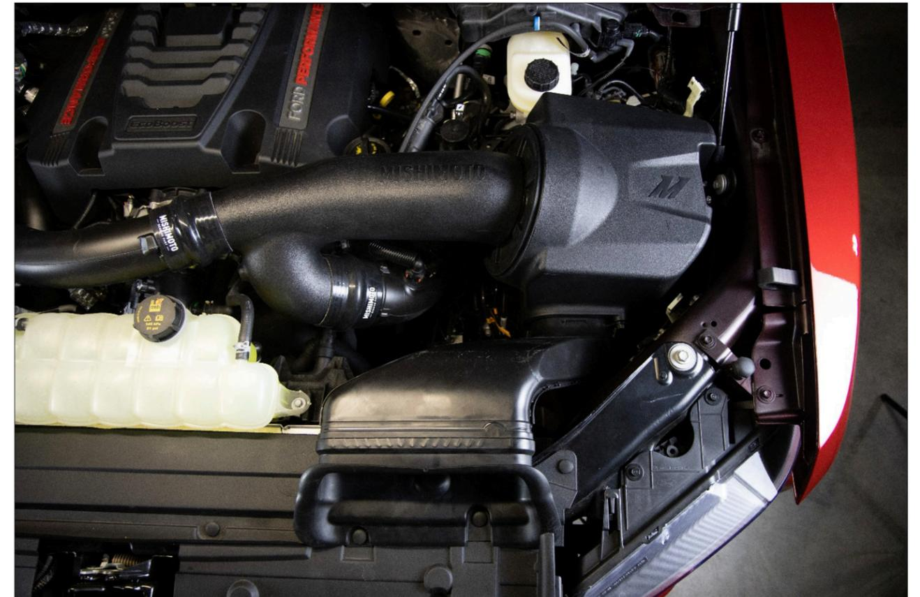
**FIGURE 2:** Mishimoto intake production sample installed on a Raptor model.
