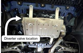
2) Remove the two hoses from in front of the diverter to gain access to the clamps behind.
