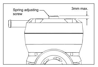
The recirc versions of the Mach 2 are supplied with GFB's softer spring (part # 6116), which cannot be used for atmosphere venting because the piston will usually hover slightly open at idle (similar to the factory valve).
