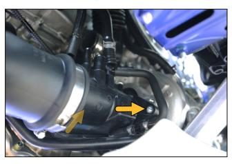
3) Using a 10mm socket, remove the two bolts that hold the turbo intake pipe onto the turbo.
