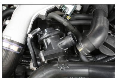
4) Fit the GFB Mach 2 valve to the intercooler, making sure the supplied red o-ring is fully inserted into the groove in the underside of the GFB valve as shown below. Replace the two bolts, vacuum and recirc hoses and clamps.
