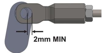
4. At this setting, it is likely that the "gate" boost pressure may be slightly under the rated spring pressure. Typically, a pre-load of 4-6mm achieves the rated spring pressure. You can adjust spring pre-load via the turnbuckle without removing the clevis from the wastegate flap - each full turn adjusts the pre-load by 2mm. Once you have set the adjustment, tighten both locknuts (remembering that the locknut closest to the WGA body is a left hand thread).
