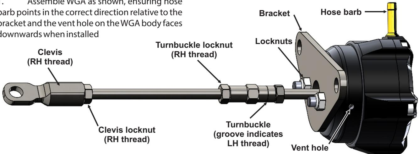
2. Ensure the clevis and turnbuckle have at least 5mm of thread engaged, but do not tighten any of the locknuts at this stage
