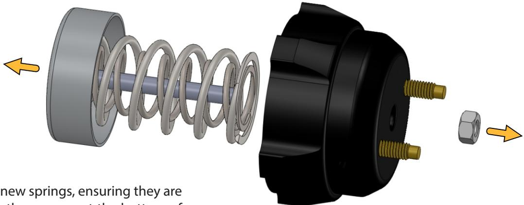
5. Install the new springs, ensuring they are correctly seated in the grooves at the bottom of the body, and on the underside of the piston
