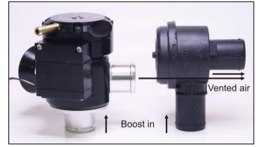
For typical Bosch diverter valve replacements (image shows a VW Golf GTI):
