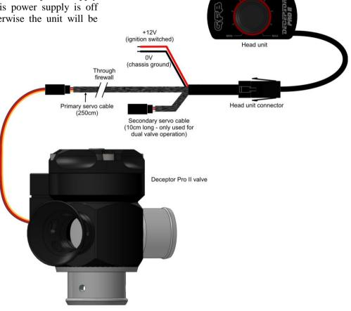
Often there is an existing grommet that can be used for this purpose. In any case, it is important to ensure that the lead is protected where it passes through the firewall to prevent wear or damage.
