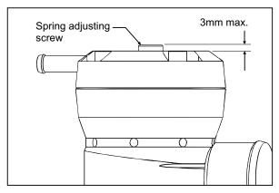
need to be adjusted to prevent stalling or backfiring, since all of the vented air is recirculated.
