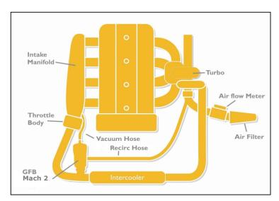
NOTE: GFB recommends mounting the valve closer to the throttle body rather than the turbo, since some factory turbo piping can cause pressure drops which may affect the performance of the valve. If an intercooler is used, it is preferable to mount the valve after the intercooler, before the throttle.
