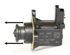
Pull on the plastic diaphragm shroud, the whole assembly will pop off leaving the bare solenoid coil. Keep the yellow o-ring.
