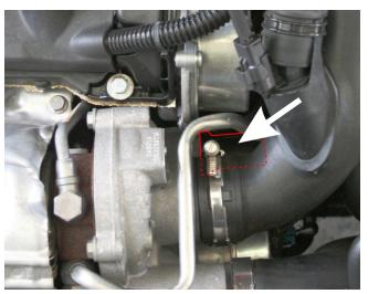
Remove the intake duct to gain access to the diverter valve and the 3 bolts holding it to the turbo. Unclip the wiring connector from the top of the solenoid coil – note there is a small locking tab that needs to be unclipped as you pull on the connector.
