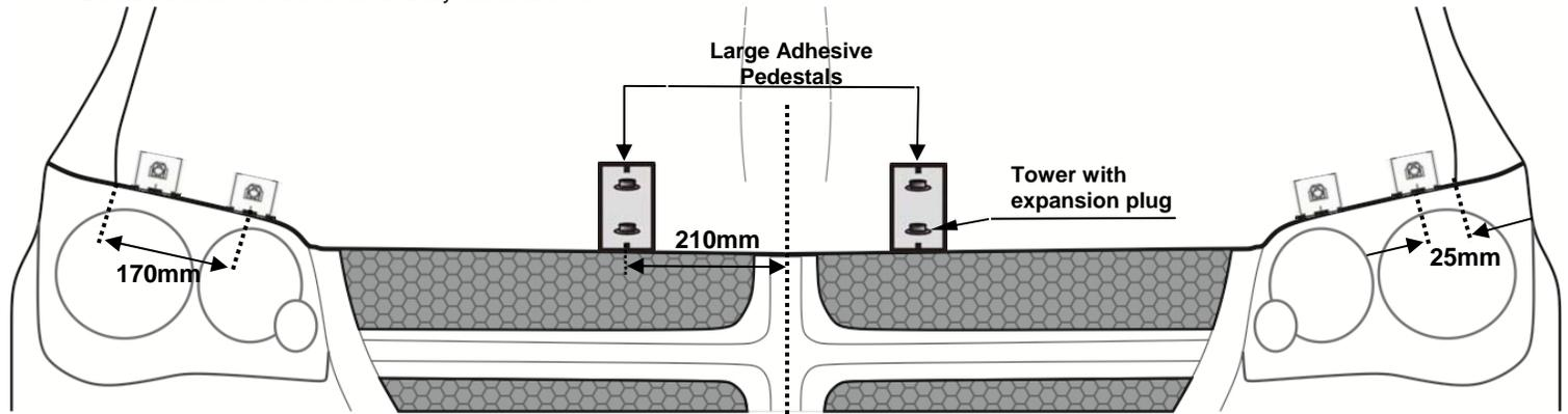
2. Install the square expansion plugs into the top of adhesive backed pedestals.
