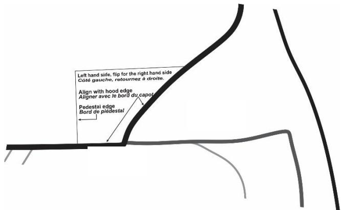
2. Cut out and tape the "Pedestal locating template" (found on page 6) to the left hand edge of the of the hood as shown.
