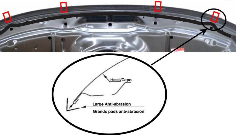
7. **⚠** Peel protective backing from the large anti-abrasion pads and wrap them around the leading edge of the hood aligned above the expansion plugs installed in step 6. See illustration
