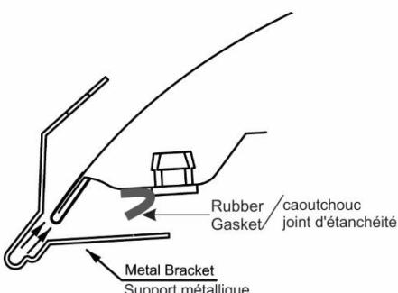
8. Install metal brackets over the hood edge in their corresponding positions making sure to install lower leg of brackets underneath the rubber gasket and aligned with the round hole in the expansion plug. See *Illustration*.
