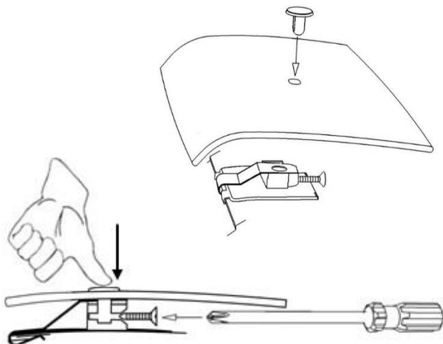
14. At the 2 outermost locations, install a pin through the protector and into the pedestal.
