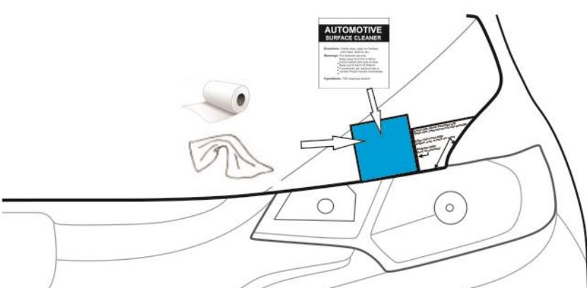
3. Using the automotive surface cleaner, 1st thoroughly wipe the shaded area of hood surface shown in the illustration followed by drying with a soft cloth or paper towel. This will insure all wax, finger prints and oils are removed from the hood surface in the bonding area.
