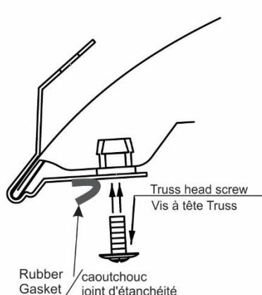
9. Loosely install truss head screws through the metal brackets and into the expansion plugs, making sure the brackets are well seated against the edge of the hood. See *Illustration*.
