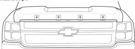
5. Temporarily tape the pedestals to surface of the hood in their determined positions. Confirm correct placement by placing the hood protector on top of the four pedestals. When positioned correctly the four (4) holes in the center area of the protector will align with the holes in the expansion plugs. Adjust if necessary and reconfirm the pedestal locations using the measurements in the illustration and the hood protector.
