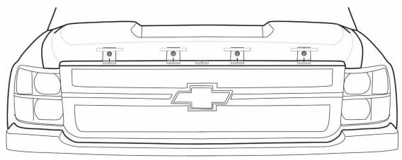
6. Using masking tape or the repositionable tape strips, outline each pedestal as shown. This will aid in placement after cleaning. Remove the pedestals and clean the contact area with the automotive surface cleaner. Dry with a soft cloth or paper towel.
