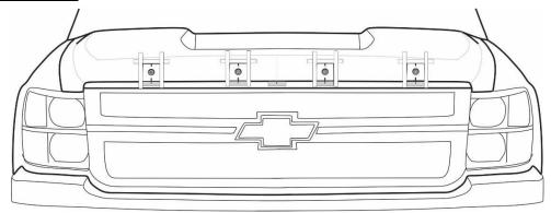
7. Remove the protective film from the bottom of the pedestal and adhere to the hood surface by contacting the leading edge of the pedestal with its location at the back of the grill surround and rotating into place on the hood surface. We to out+surface of the pedestal to ensure complete contact of the adhesive with the surface of the hood. See Illustration.
