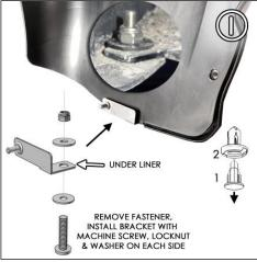
**FIGURE J** Install Stainless Steel Screw 1SS and Small Washer SMWASH through mud flap then through a Round Plastic Spacer .25SP and Foam Spacer for top 2 mounting points. TIGHTEN ONLY UNTIL MUD FLAP IS LEVEL WITH BUMPER. Do not fully tighten.
