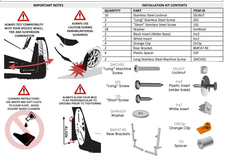
**Recommended Tools** Low-profile, ratcheting offset or stubby Phillips screwdriver, small flathead screwdriver, pick, 7/16<sup>°</sup> wrench, panel removal tool. **Important Tips** Installation should be done on an even surface. The hardware self-threads so avoid overtightening.
