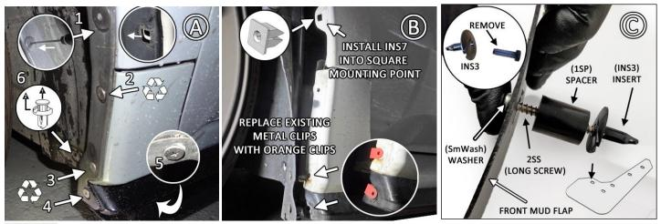
**FIGURE D** INS3 Insert assembly goes into mounting point 6. It should be firmly seated against the liner. Hold female base portion of insert securely against liner to prevent it from spinning. Continue threading the Long Screw (2SS), keeping the Insert seated against liner during this process. Tighten until washer is *almost* seated against the flap. Do not fully tighten so you can adjust later.
