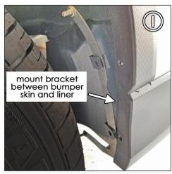
FIGURE J Install factory push fastener exterior housing through the bumper and Rear Bracket then use the interior pin to lock in. To align, lower Rear Bracket can be adjusted by hand.
