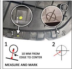
FIGURE J Using a small bit, drill a pilot hole in the center of the marks.
