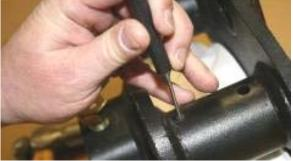
3. Install the new retaining spring and drive screw. Be sure to insert the retaining pin into the top hole of the head. Insert new drive screw into bottom and gently tap into place with a hammer.
