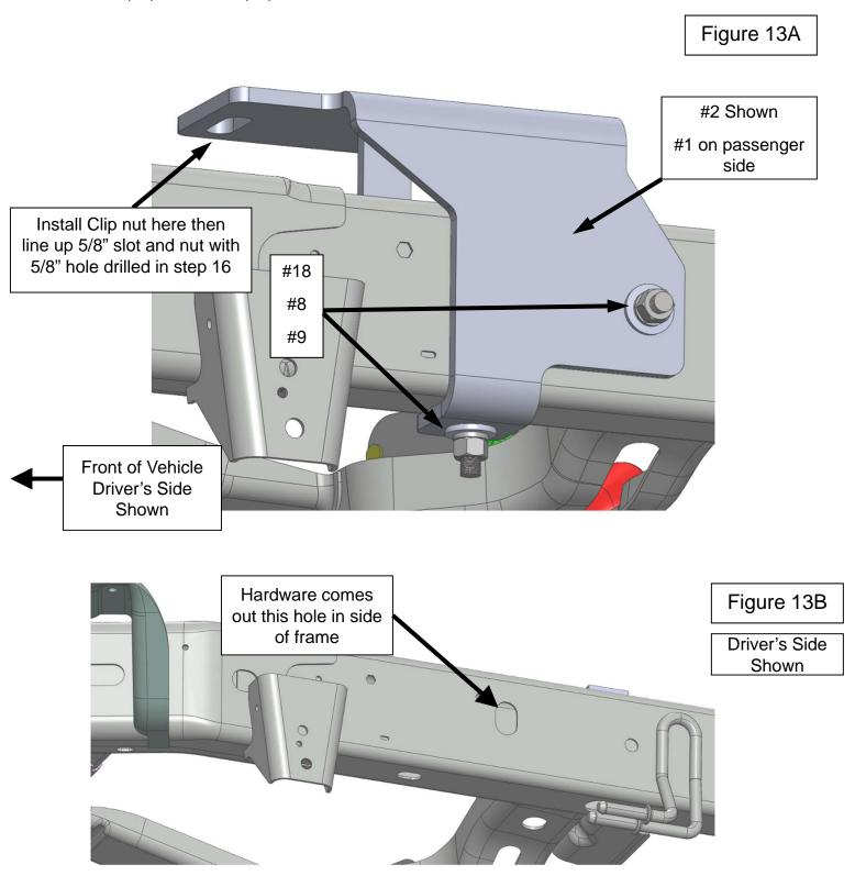
16. Align the rear base rail with the holes drilled in steps 16. Use the 5/8" Hex head bolts (#14), 5/8" flat washer (#15) & 5/8" Lock washer (#17) to attach the rear base rail to the rear brackets installed in step 16. Remeasure your base rails as in Step 2. Once you are sure everything is square; hand tighten the 5/8" hardware first. Then tighten and torque the ½" hardware on the rear brackets to 75 ft. lbs.
