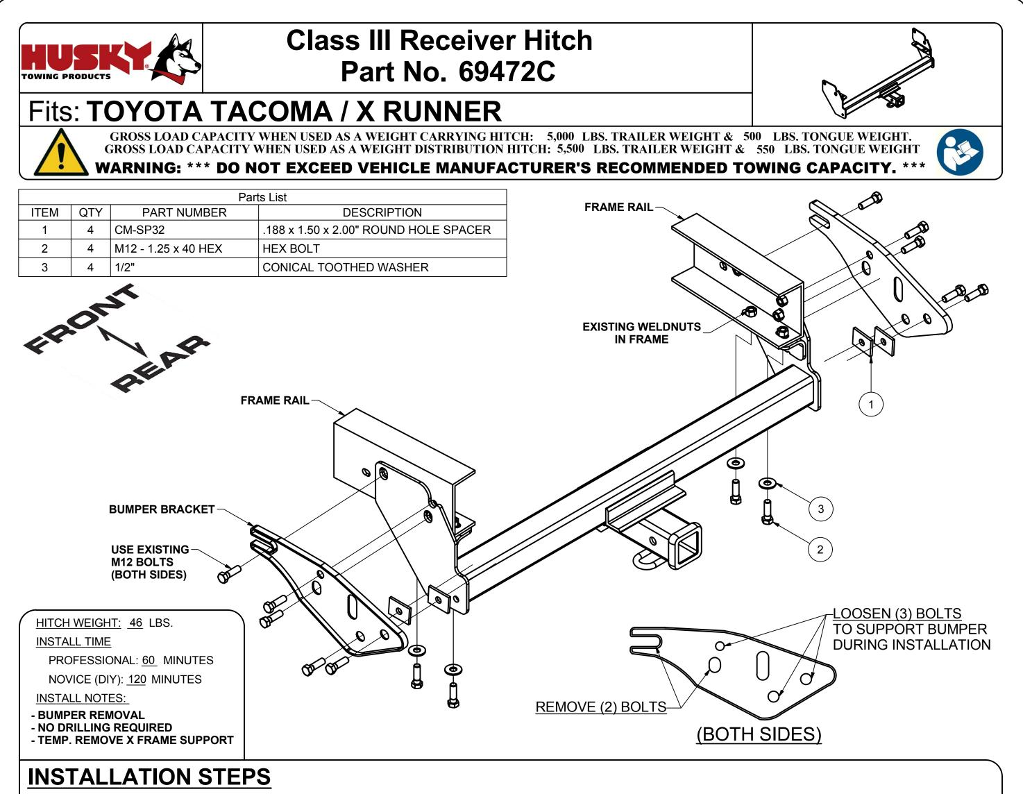
If bumper alignment pin interferes with hitch installation, use a saw or cutoff wheel to remove the alignment pin from the side bracket.\*\*
