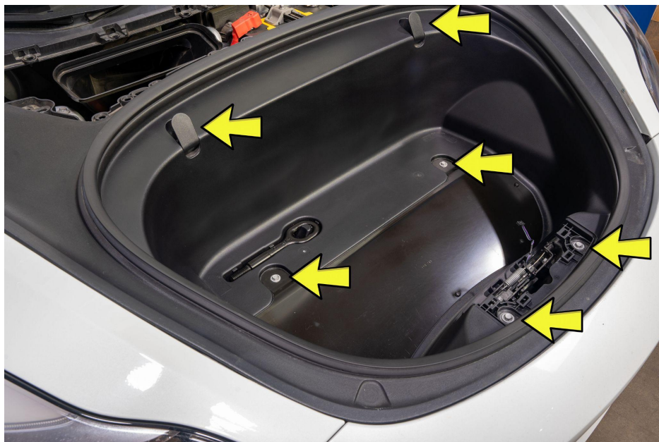
7. Use a 10mm socket and remove the 6 bolts from the frunk storage compartment tub. Remove the frunk storage compartment tub.
