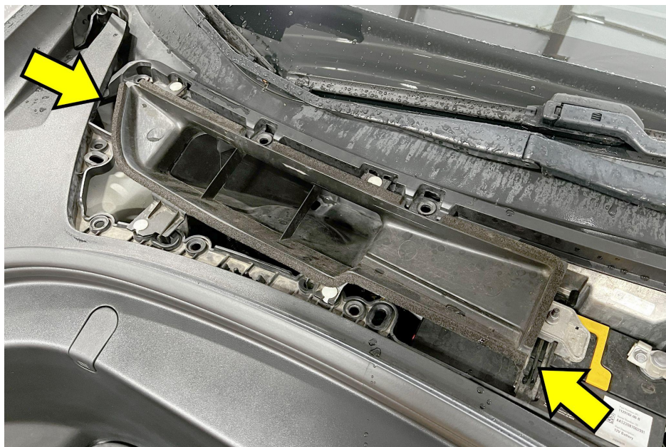
3. Pull up to remove the cabin air inlet duct.
