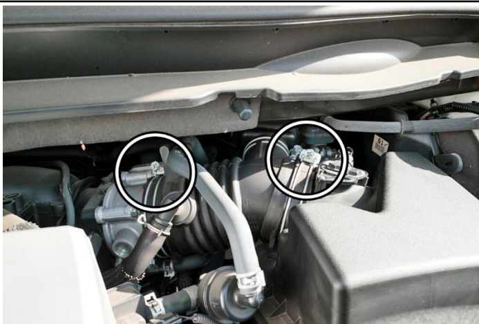
2. Loosen the hose clamps securing the factory intake hose from the throttle body and the air box.
