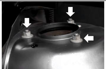
4. Remove the 3 nuts on each of the strut towers. If stock, use a 13mm socket.
