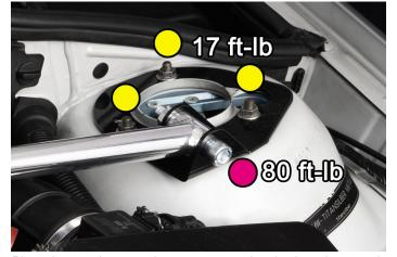
5. Place the strut bar onto the strut tower using the 3 studs on each side to align it into place. Reinstall the 6 nuts that were removed and fasten to 17 ft-lb. Fasten the hardware between the bar and bracket using a 10mm allen key and 18mm wrench and torque to 80 ft-lb.
