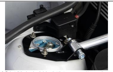
6. Reinstall the hood switch bracket that was removed in an earlier step.
