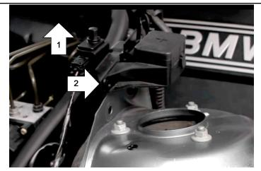
3. Lift up on the hood switch bracket (1) and push the plastic rivet out towards the front of the vehicle (2). Carefully lift the switch/battery terminal assembly up enough to let the strut bar bracket fit underneath.
