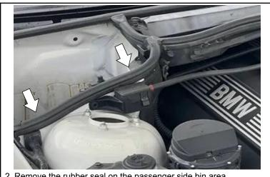
2. Remove the rubber seal on the passenger side bin area.
