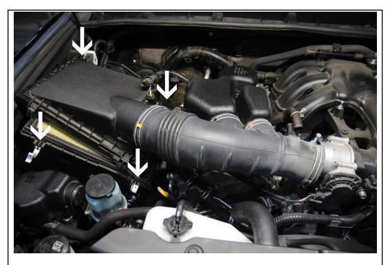
3. Unclip the 4 clips that hold the upper intake box in place. Move the intake box up and over to the side so that there is space to remove the OEM intake.
