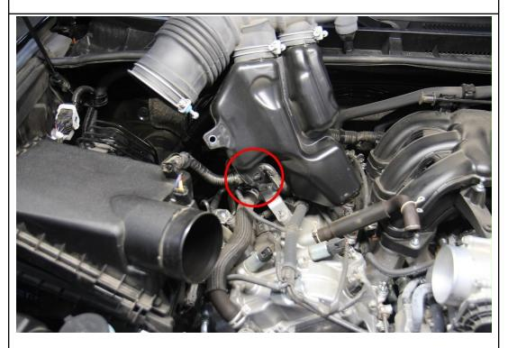
4. Flip the stock intake so the MAF harness clip is exposed. Use a flat head screwdriver to unclip the harness from the resonator and remove stock intake assembly.
