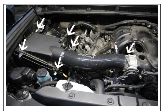
5. First, install the HPS silicone tube onto the throttle body with the provided T-bolt clamp SSTC-86-94, then onto the stock air box outlet with the provided T-bolt clamp SSTC-102-110. Attach the stock air box back in place and fasten the 4 clips.
