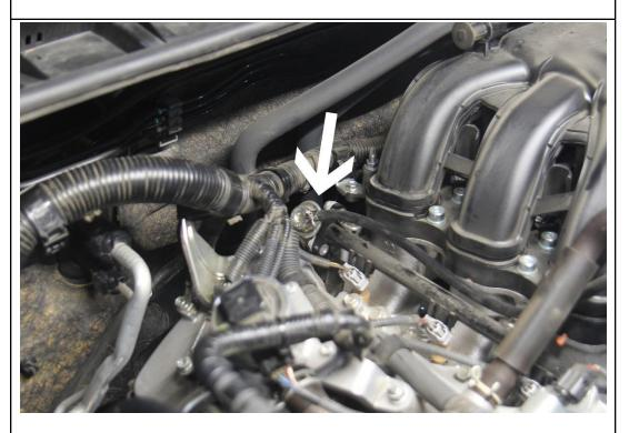
6. Remove the stock vacuum hose from the fuel pressure regulator and replace it with the HPS vacuum hose, part number HTSVH4-BLK, then secure the vacuum hose with the provided FIC-8 clamp.
