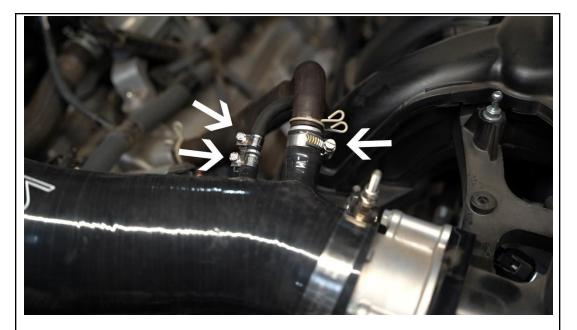
7. To install the vacuum hose, slip the clamp FIC-10 onto the intake then install the vacuum hose onto the intake barb with the clamp FIC-8. To install the PCV hose, slip the EMSC-16-27 clamp onto the intake then install the PCV hose back onto the intake barb.
