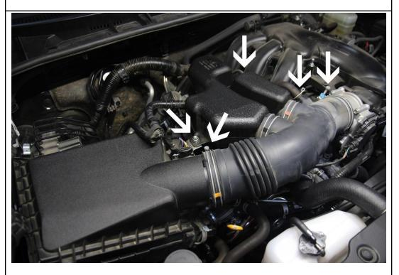
2. Loosen the intake clamps at the throttle body and the air box. Disconnect the PCV hose located next to the throttle body on the intake. Disconnect the vacuum hose located behind the intake resonator. Then, remove the 10mm bolt to disconnect the intake resonator mount.
