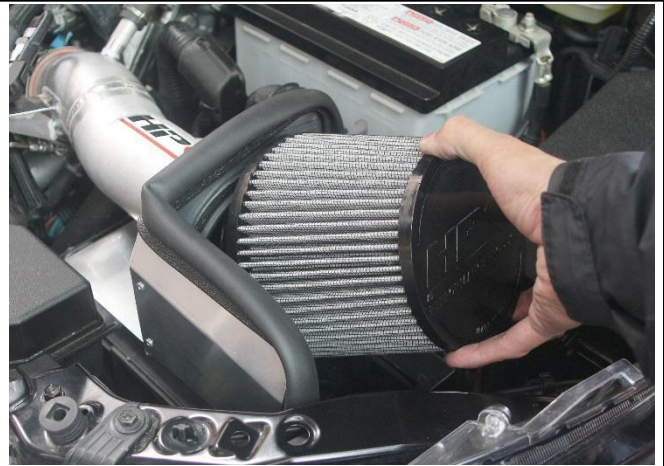
37. Insert the HPS air filter through the heat shield opening and onto the intake pipe.
