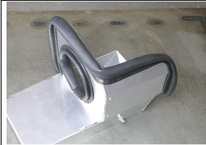
16. Once the stretching is done, you can continue to install the edge trim along the remainder of the heat shield.
