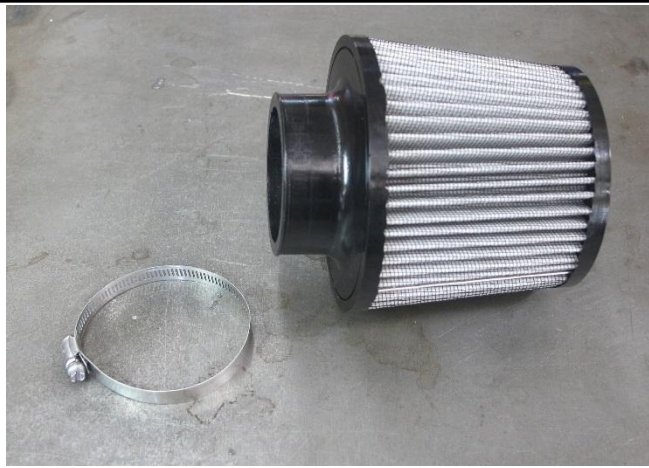
34. Separate the hose clamp from the air filter.
