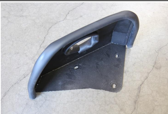
8. Install the provided bubble edge trim onto the heat shield.
