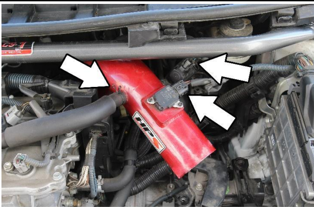
6. Insert the factory breather hose onto the intake pipe, then reinsert the factory MAF sensor harness and the EVAP sensor harness.
