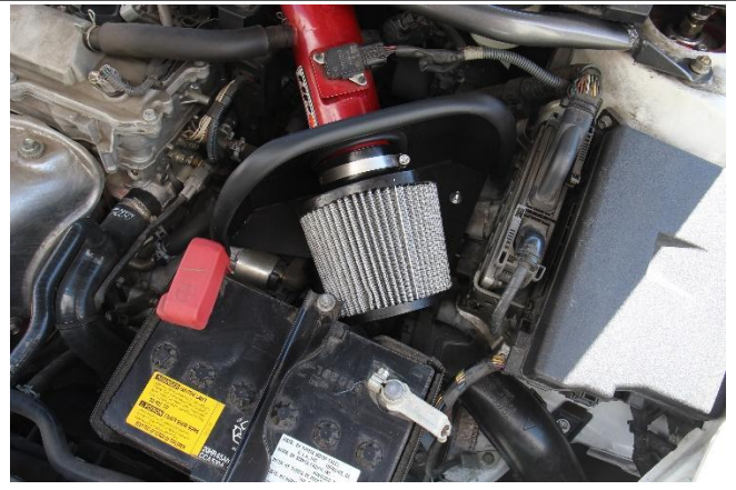
11. Install the provided HPS performance air filter.
