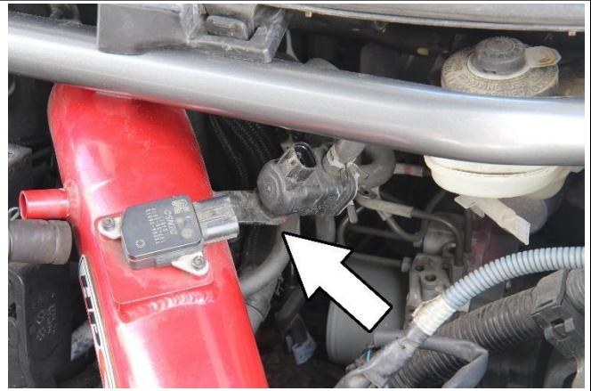
5. Insert the intake pipe onto the throttle body coupler. Reinstall the factory EVAP sensor onto the intake pipe using the factory screws and secure the MAF sensor using the provided 4mm allen head screws.
