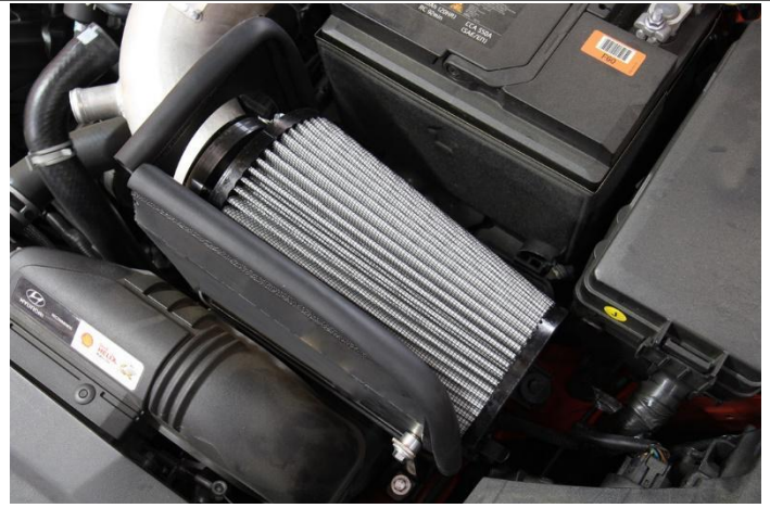
17. Insert and secure the HPS performance air filter onto the HPS intake pipe.
