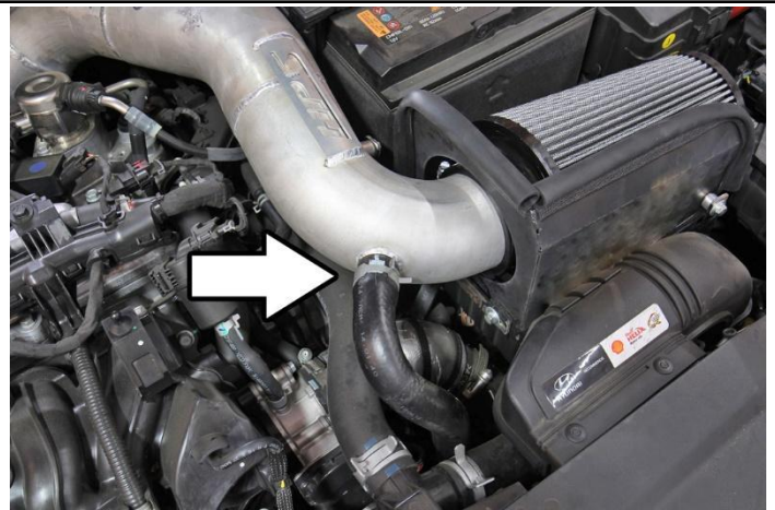
19. Reconnect the recirculating valve hose onto the intake pipe.
