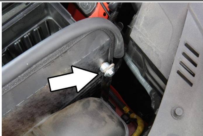
14. Secure the "L" bracket to the heat shield using the provided spacer in between the bracket, M6x25mm bolt, and washer.
