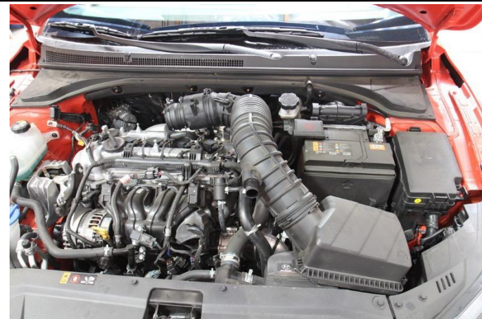
6. Remove the entire intake tube and the upper air box assembly from the vehicle.
