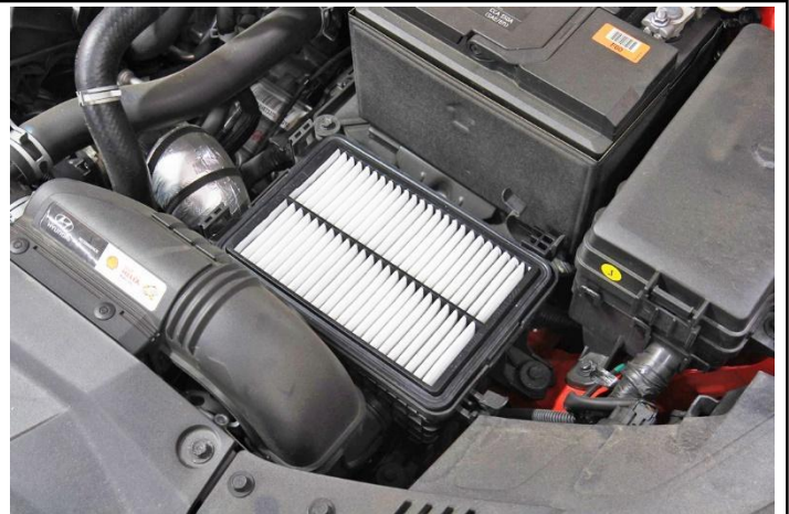
7. Remove the air filter from the vehicle.
