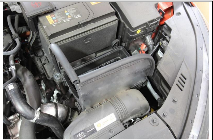
11. Place the heat shield onto the lower air box assembly.
