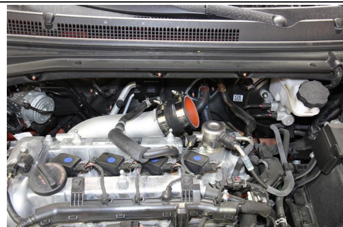
8. Install the reducer coupler along with the provided T-bolt clamps onto the turbo inlet.
